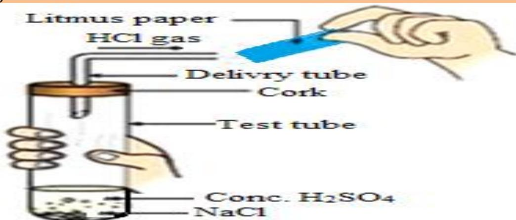
Blue litmus paper is brought near the mouth of the delivery tube to check the presence of HCl acid but no change is observed in the color of litmus paper because:
